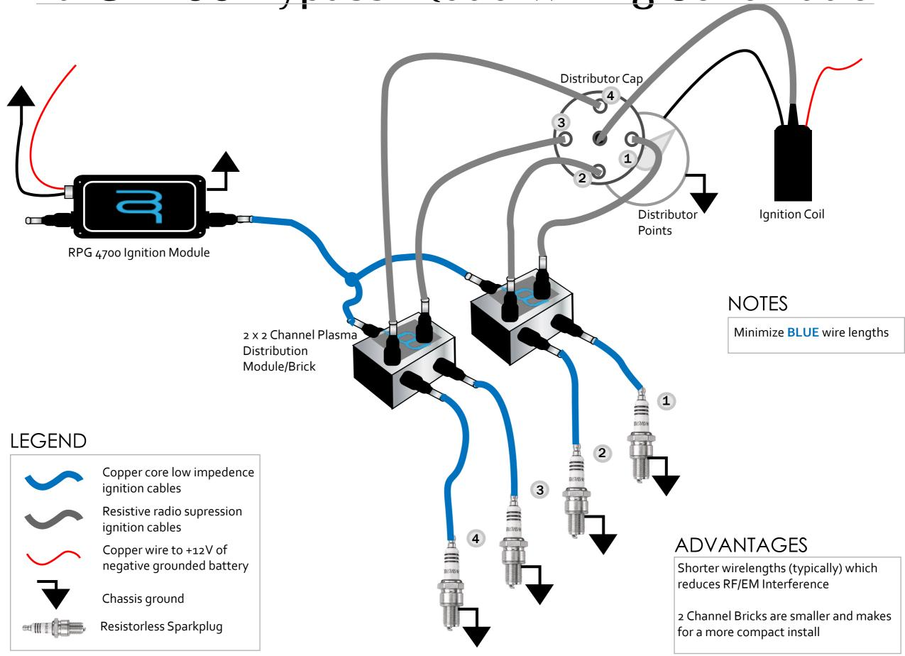
RPG 4700 Bypass Mode Wiring Schematic Distributor Cap Distributor Ignition Coil **Points** RPG 4700 Ignition Module 4 Channel Plasma Distribution Module/Brick LEGEND Copper core low impedence ignition cables Resistive radio supression ignition cables Copper wire to +12V of negative grounded battery **NOTES** Chassis ground Minimize **BLUE** wire lengths
